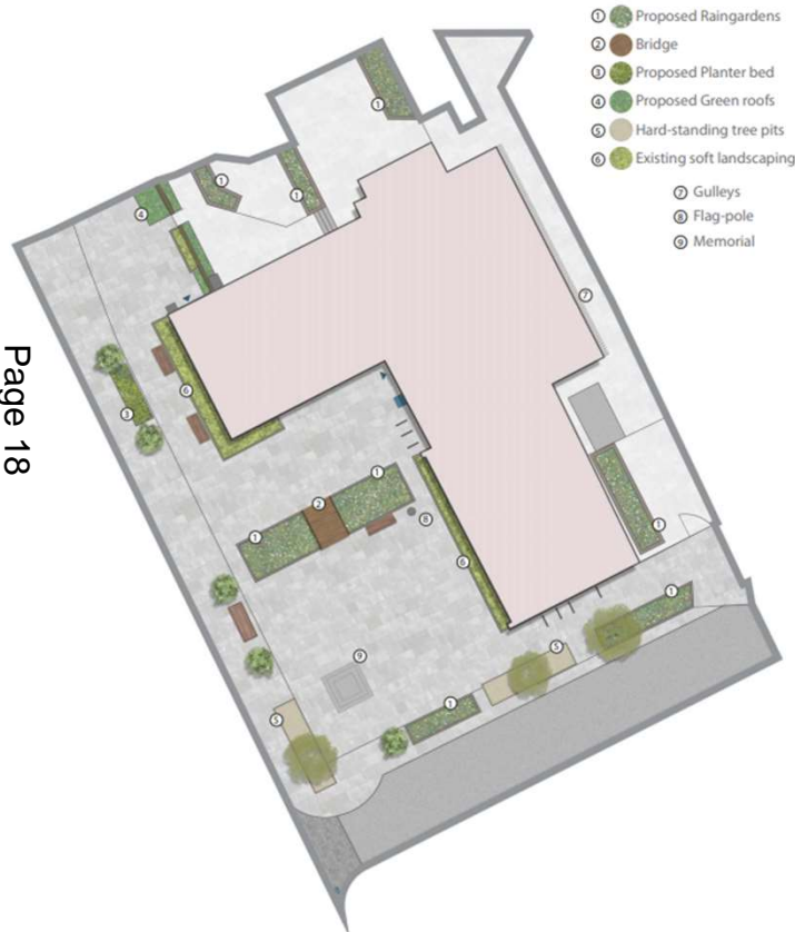
1 Rain gardens - SuDS that capture rainfall before it enters the piped network and allows it to infiltrate into the ground.
